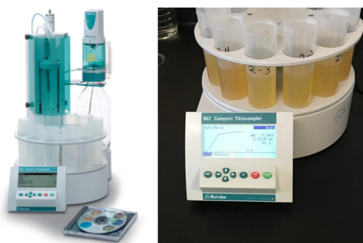
Figure 2.4: Automatic multiple positions titrator (862 Compact Titrator, Metrohm AG, Switzerland) for the TA determination expressed as malic acid equivalents.
