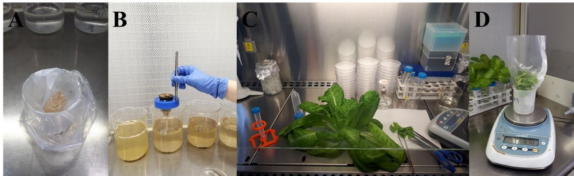
Figure 4.S1. Root rinse collection (A), root sterilization (B) and leaf sampling procedure (C, D).
