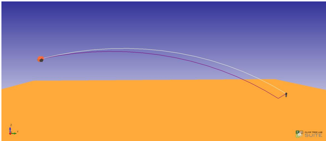
Figure 22. Refracted paths from moderate positive diffraction.
