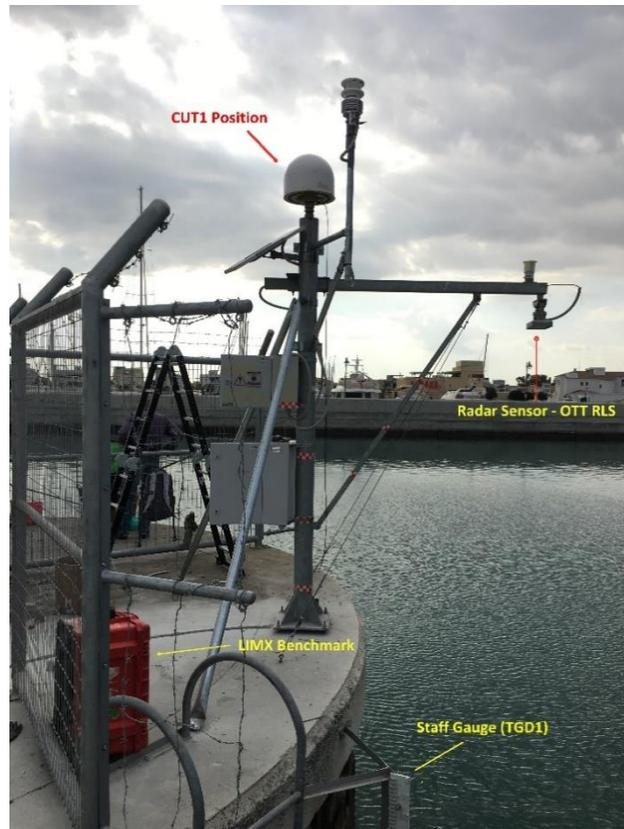
**Figure 2.** The Limassol (LEME) integrated tide gauge station.
