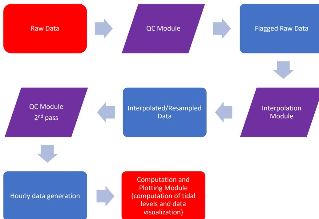
Figure 6. The processing workflow for the determination of tidal levels.
