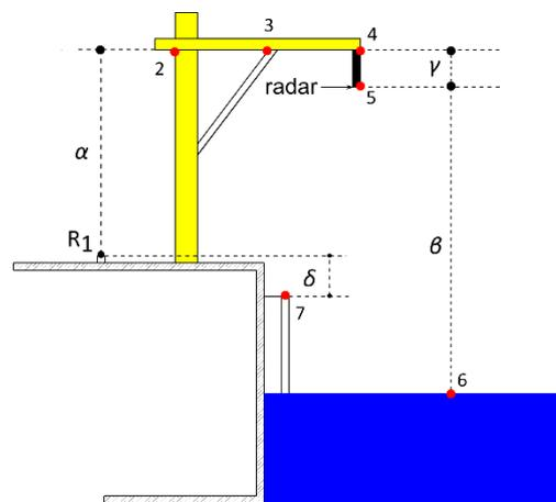
**Figure 5.** Tide gauge significant control points and their offsets.
