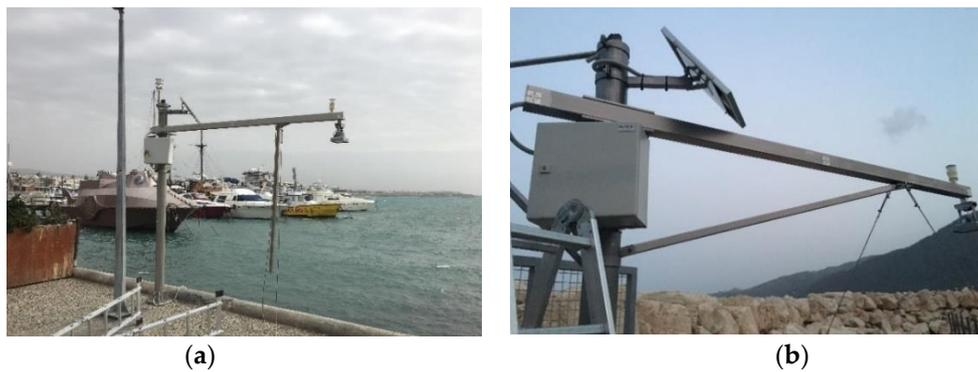
**Figure 4.** (a) the tide gauge horizontal mast during maintenance, (b) the installation of special adhesive targets along the mast to check alignment.
