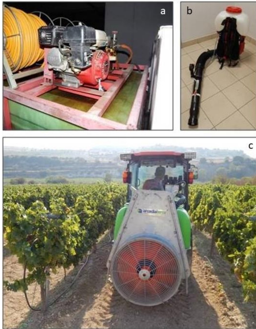
Figure 6: Sprayers tested: a) HVS with a spray gun b) LVS (Motorized knapsack sprayer) c) OS (Axial fan orchard sprayer)
