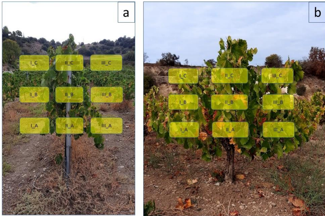
Figure 17: Water sensitive paper's positions for a) Trellis trained vines b) Goblet trained vines
