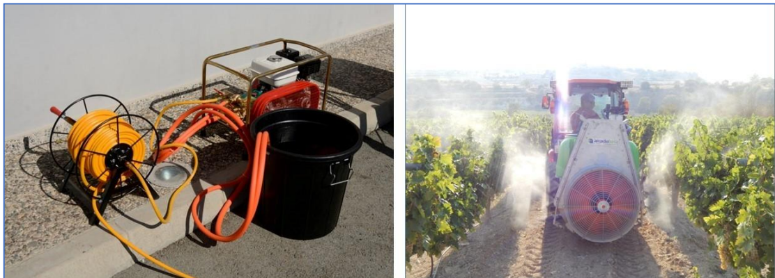
Figure 16: Sprayers tested. On the left the HVS with the spray gun and on the right the orchard sprayer used for the OS500 and OS250 treatments.
