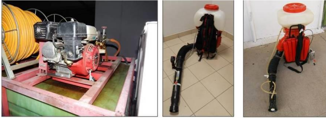
Figure 1: Sprayers tested from left to right: 1) High Volume Sprayer with spray gun (HVS) (Honda GX 120, 4.0 HP), 2) Motorized air assisted Low Volume knapsack Sprayer (LVS) (CIFARELLI, Mist Blower M1200), and 3) Common knapsack Sprayer (CS) (Dinyi, Model 3WF-3, JAPAN)
