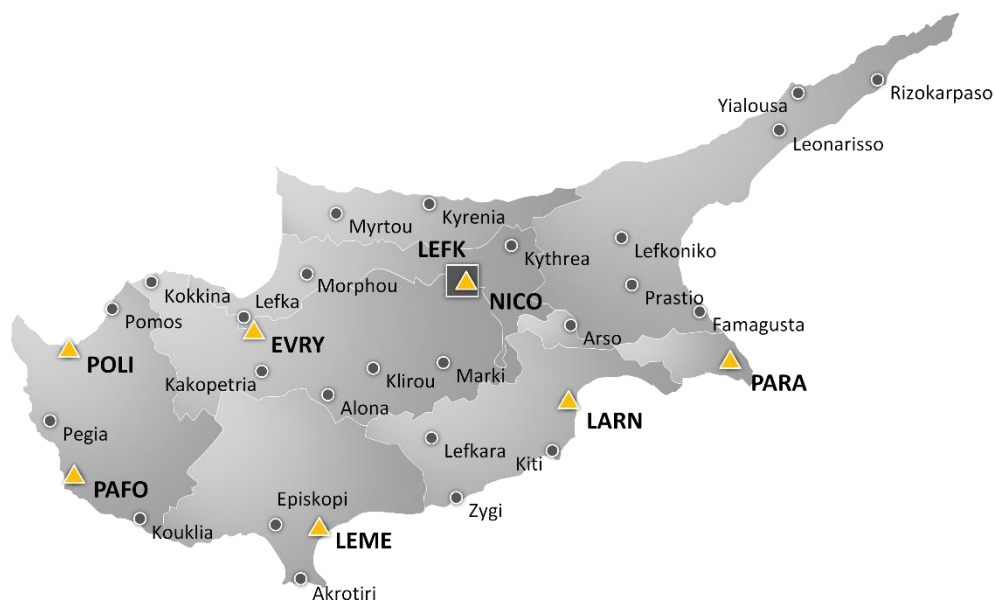
Figure 52: The CYPOS permanent GNSS network
