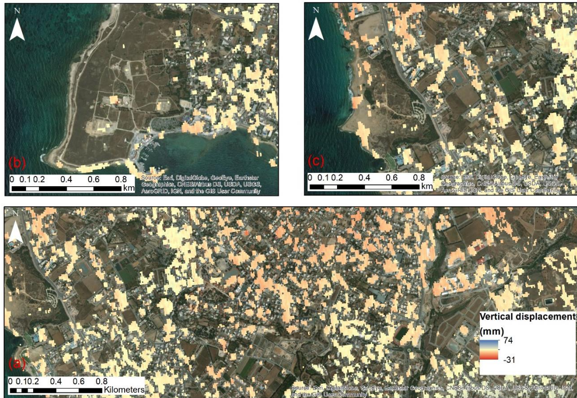
Figure 68: Final displacement map at (a) historic centre of Paphos; (b) Nea Paphos and (c) Tombs of the Kings
