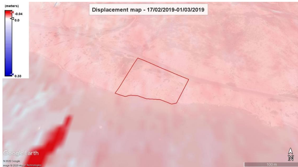
Figure 80: Displacement maps at the landslide area near Petra tou Romiou
