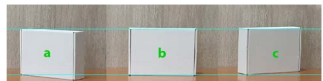
Fig. 5. Photos of a rectangular object in the vertical position. (a) and (c) When viewed at an angle it always shows a smaller width, in this case 2.3 units in (a) and 2.2 units in (c). (b) viewed from the front, it registers its correct width (2.8 units).
