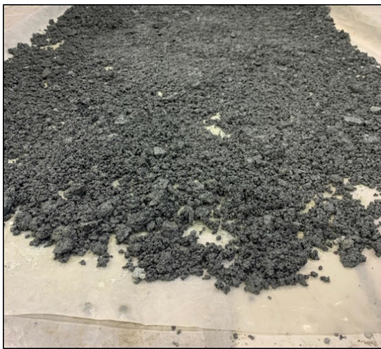
Fig. 2. Coated rubber particles on plastic sheathing.
