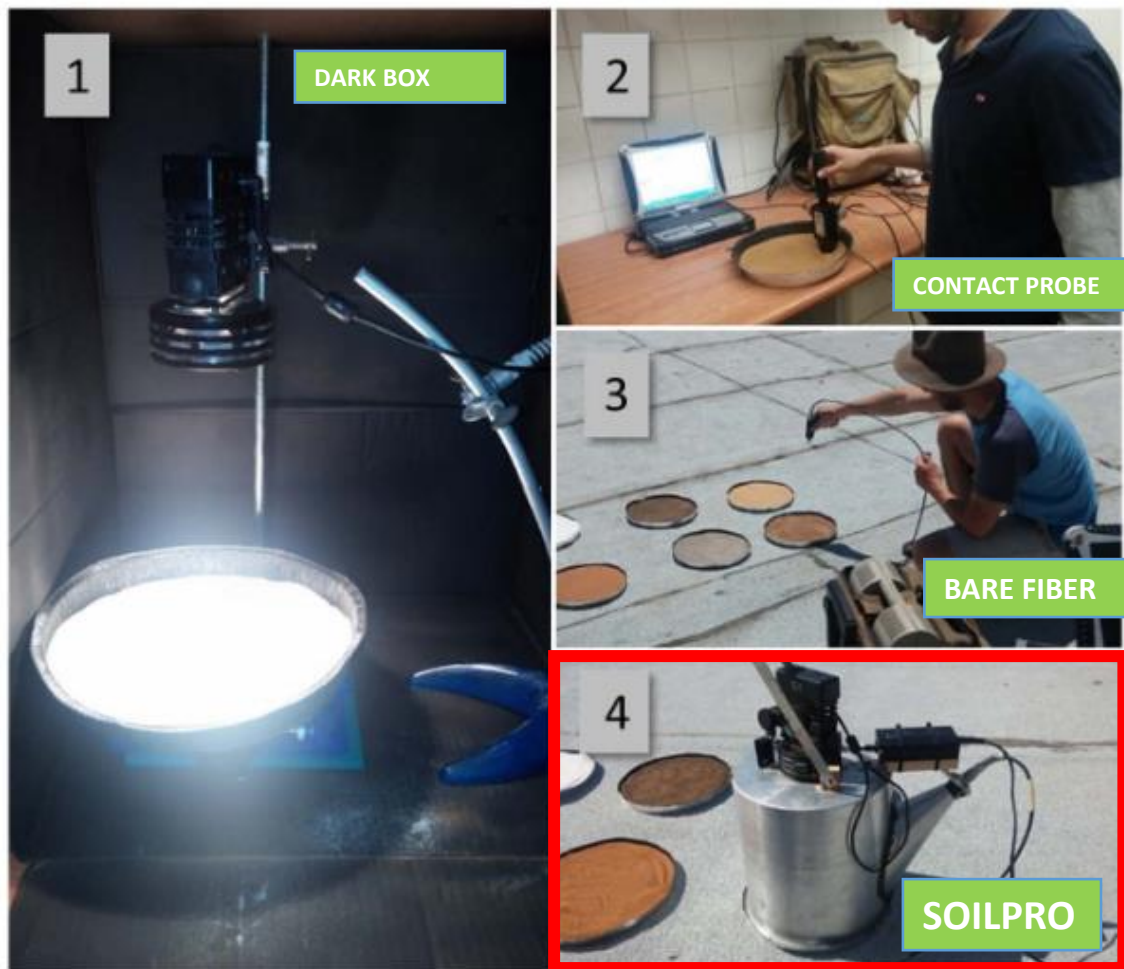
Fig. 3. Measurement procedure. (1) Bare fiber in the laboratory in dark box configuration, the lamp points downward toward the targets at nadir while the fiber tip points at 45° from the calculated distance according to the fiber FOV, to view most of the target. (2) Contact probe in the laboratory. (3) Bare fiber outdoors. (4) SoilPRO outdoors.
