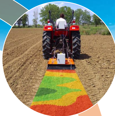
Mobile Soil Sensor System [vis-NIR Spectrometer]
