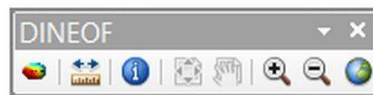
Figure 6.5: DINEOF toolbar in ArcMap. Button icons description (from left to the right): Main process button, distance measure button, information button, copy and paste buttons, zoom and pan buttons, view entire region button.
