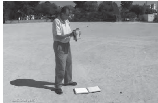
Figure 2: Collection of spectral signature data on a whitish bare soil using the GER1500 Field Spectroradiometer
