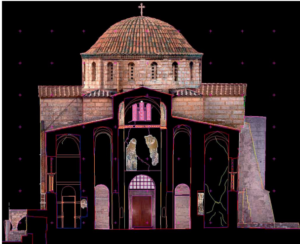
Fig. 1 Combination of vector restitution and raster orthoimages: vertical section of Byzantine church of Dafni (Greece), where the internal mosaics are shown.
