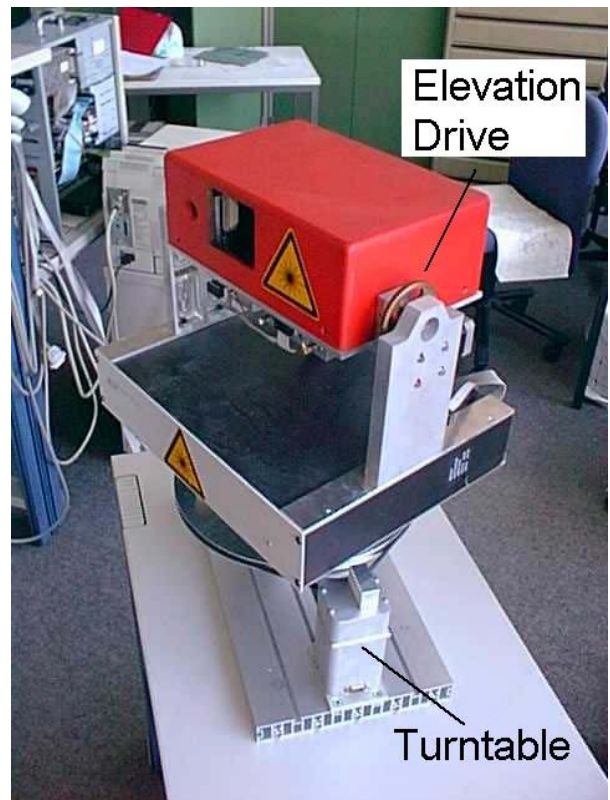
Figure 4. 3D-LS on Turntable
