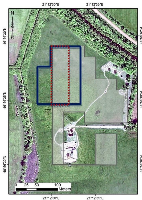
Figure 1. Area covered from the different techniques: Grey and blue polygons indicate the areas covered from the geophysical surveys (magnetic and GPR survey, respectively), the red polygon indicates the area covered from the ground spectroradiometric measurements (Latitude: 46^{\circ}56'24.36'' ; Longitude: 21^{\circ}12'32.67'' ) (source [26]).
