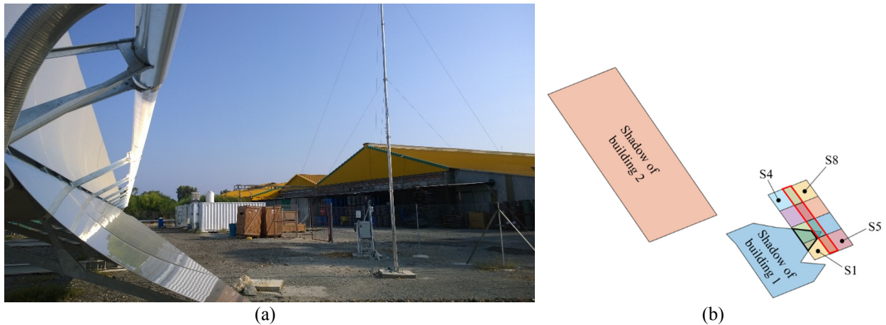
FIGURE 4. (a) PTC in the vicinity of buildings and trees (© Protarget). (b) Computed shadow area polygons for building 1 and building 2. Computed shadow area polygons of collector row 1 (12 metre segments S1 to S4) as well as collector row 2 (segments S5 to S8). The area encompassed by a thick black line is the shadow area cast onto collector 1 by building 1. The area encompassed by the thick red line represents the shadowing of collector row 1 onto collector row 2. (© SIJ)
