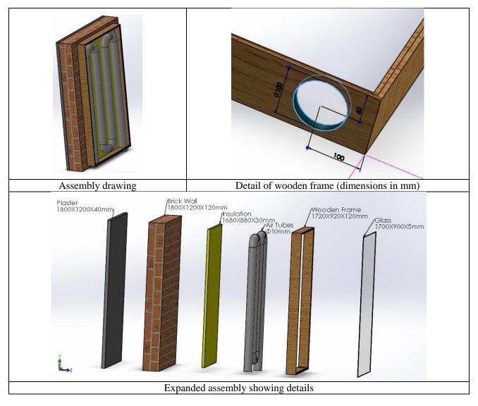
Figure 1. Integrated hot air collector utilising an aluminium foil duct
