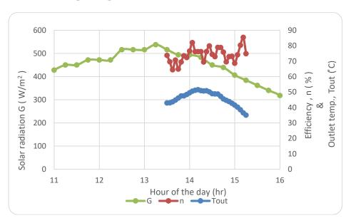
Figure 8. Efficiency of the integrated hot air collector with internal metal separators, varying during the testing period, from a minimum of 63 to a maximum of 82%.
