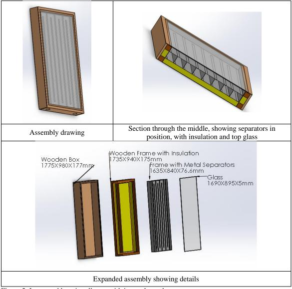
Figure 2. Integrated hot air collector with internal metal separators
