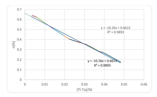
Figure 7. Efficiency of the integrated hot air collector utilising an aluminium foil duct, with a fun speed of 1.9 m/s and an incident radiation of 560 W/m<sup>2</sup>. Abbreviations: n= efficiency, Ti= initial air temperature (°C), Ta= air temperature of environment (°C), Gt= solar radiation (W/m<sup>2</sup>)
