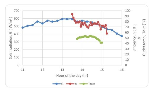
Figure 9. Efficiency of the Integrated hot air collector with internal metal separators, varying during the testing period, from a minimum of 68 to a maximum of 80%.
