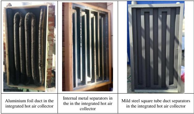
Figure 4. Duct details in the three types of integrated hot air collectors
