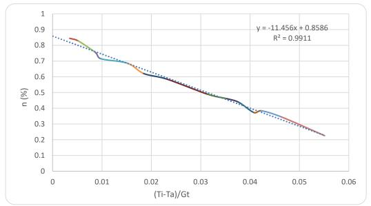
Figure 6. Efficiency of the integrated hot air collector utilising an aluminium foil duct, with a fan speed of 2.1 m/s and an incident radiation of 461 W/m<sup>2</sup>. Abbreviations: n= efficiency, Ti= initial air temperature (°C), Ta= air temperature of environment (°C), G<sub>t</sub>= solar radiation (W/m<sup>2</sup>)
