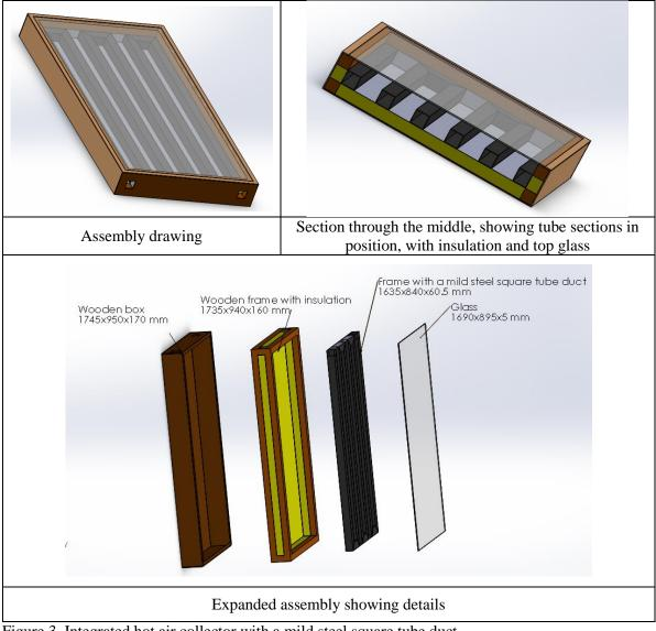
Figure 3. Integrated hot air collector with a mild steel square tube duct
