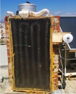
Figure 5. Pyranometer, air flow meter and temperature sensors in position for testing the performance of the integrated hot air collector utilising an aluminium foil duct.
