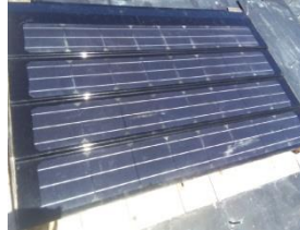
Fig.2. Picture of the module after 6 months of exposure
