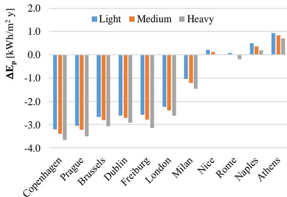
Fig. 5. HVAC system primary energy saving
