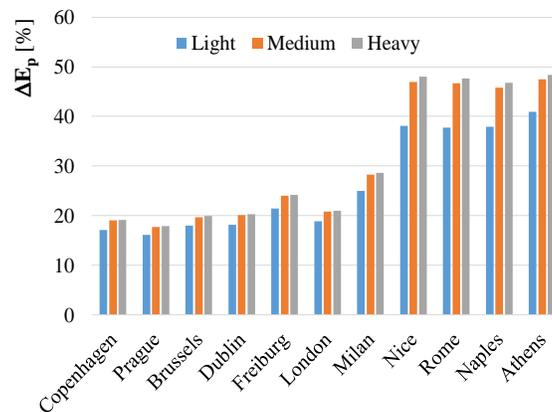
Fig. 6. Overall primary energy savings of BISTS layouts
