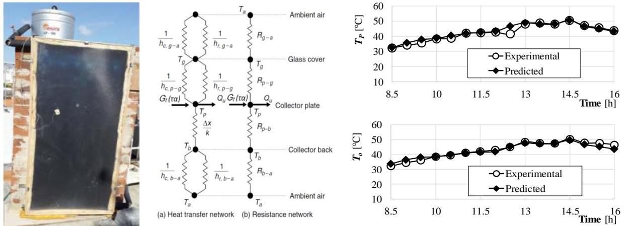
Fig. 1. FPC prototype, model thermal network and simulation/experimental results
