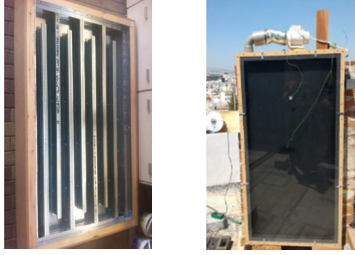
Fig. 1. Air collector prototype: internal configuration and exterior design
