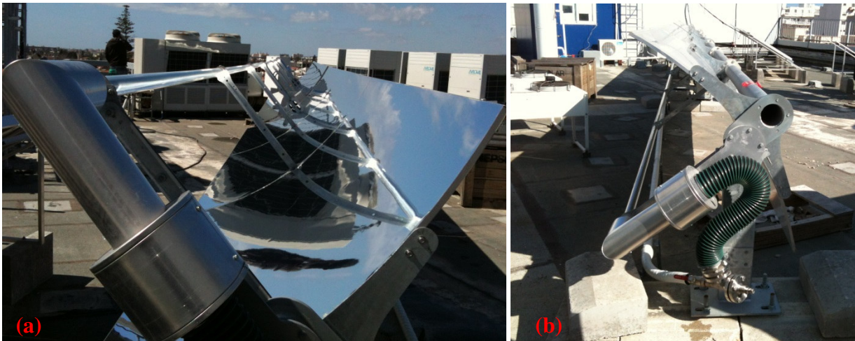
Fig. 3. Photos of the PTC (a) on focus position , (b) at park position
