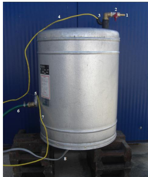
Fig. 2 Tank with PCM equipped with thermocouples to measure temperature
