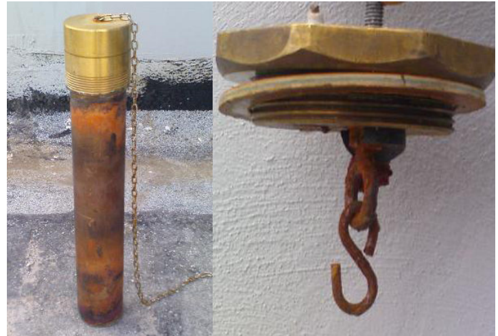
Fig. 1 Special container for the PCM and special flange used to insert the PCM-vessel in the tank.
