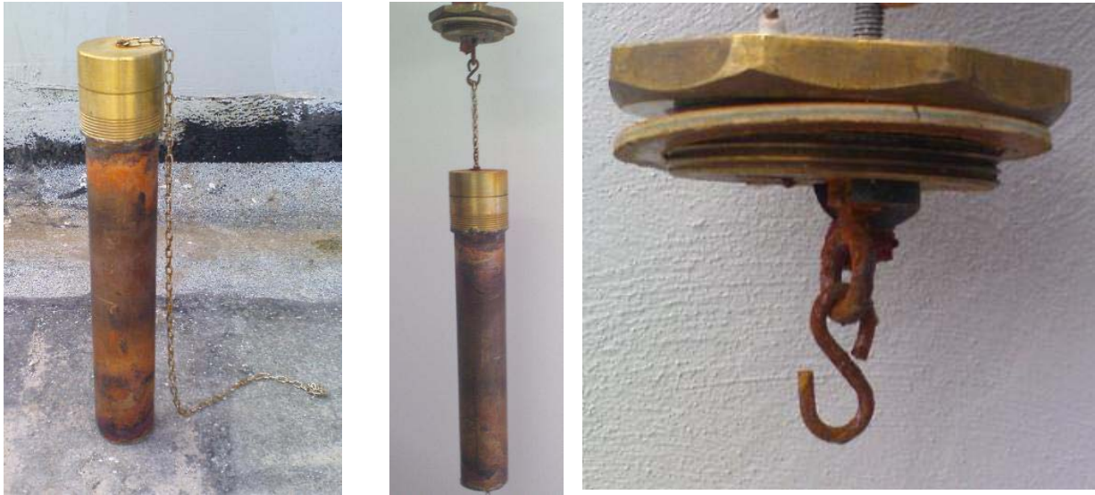
Fig. 1 Special container for the PCM and special flange used to insert the PCM-vessel in the tank.
