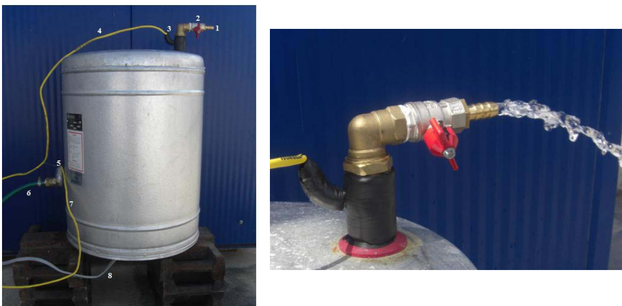
Fig. 2 Tank with PCM equipped with thermocouples to measure temperature (left) and during draw off (right)
