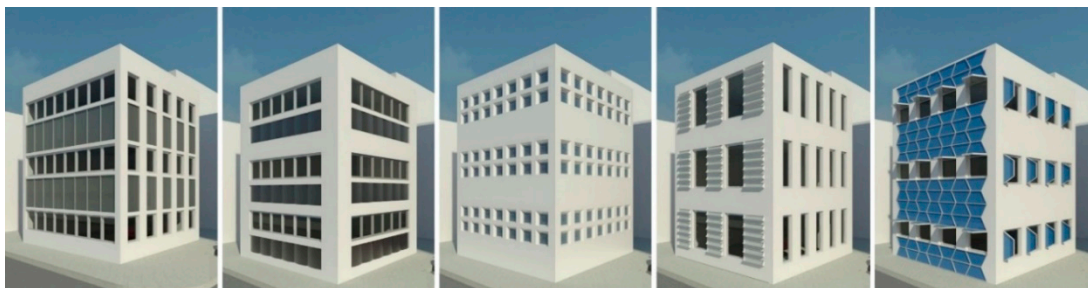
Figure 1. Visualisations of the five systems that were applied to a three-storey building. From the left: the Modular Intergrated Solar/Thermal Flat Plate Collector, the Hybrid Photovoltaic/Solar Thermal (HyPVT), the Concentrating Photovoltaic/Thermal Glazing (CoPVTG), the Solar Plenum and the Trapeze Flat-Plate Solar Thermal Collectors (FPSTC).
