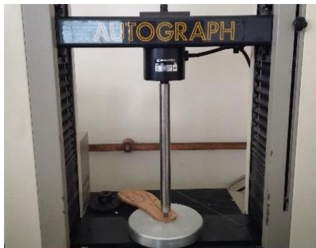
Figure 45: a) Schematic representation of the monitoring system. b) Photograph of the pressure testing platform with the cork insole.
