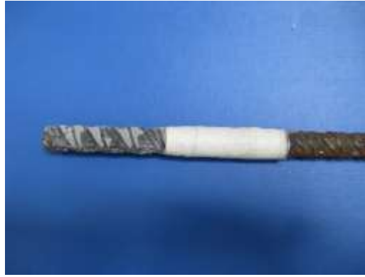
Fig.7 Steel reinforcing bar after pullout test
