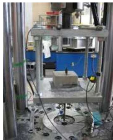
Fig.3 Test setup adopted for experiments: a) cross-sectional view of pull-out rig with specimen and instrumentation, b) smaller mounting rig with LVDTs at loaded end, c) pullout specimen testing, d) splitting specimen testing
