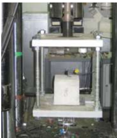
Fig.3 Test setup adopted for experiments: a) cross-sectional view of pull-out rig with specimen and instrumentation, b) smaller mounting rig with LVDTs at loaded end, c) pullout specimen testing, d) splitting specimen testing
