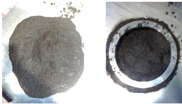
Figure 2: Slump-flow (left) and J-ring (right) testing of SFRC with 100 kg of TCF-15 per m 3 of concrete
