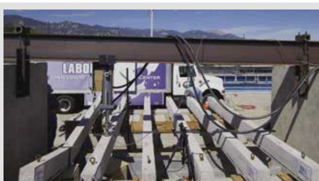
Figure 5. Beam load testing setup.
