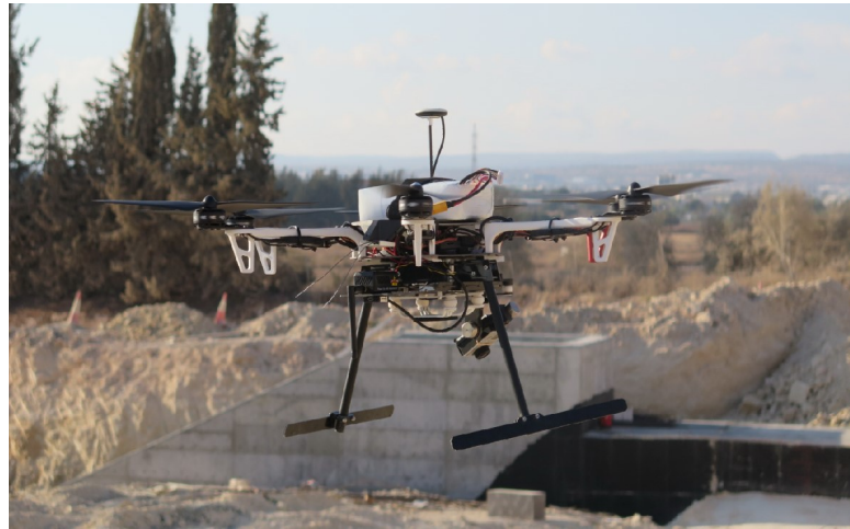
Figure 12: The UAV quadcopter with GNSS Leica Viva+ sensor with an accuracy of less than 2 cm (in 3 dimensions).
