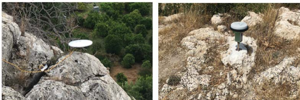
Figure 5: Trimble Zephyr 2 GNSS (left) and Leica GS15 Smart GNSS Receivers (right) for establishing a GNSS control network
