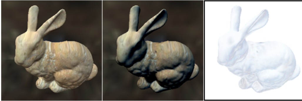
Figure 18: Self shadows are also computed at run time using precomputed FIVs. Only direct illumination without considering self-occlusions (left), direct illumination and self-shadows (middle), isolated self-shadow (right).
