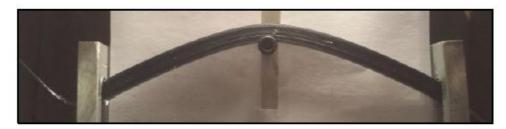
Figure 2. Bend test on the 3D printing embedded structure. The fibre is embedded near the neutral axis of the fibre
