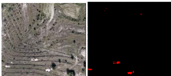
Figure 7: Simple rule base threshold values applied to the RGB bands of the orthophoto image acquired in 2014.
