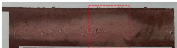
Figure 3.4: Sintered Cu structure with different focuses. Red dashed boarded area indicates the sintered area with 12-16 mm distance between focusing lense and sample surface
