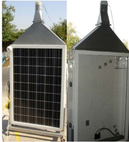
Figure 2.14. Front and back side of the test device representing a double façade with PV integration (Zogou and Stapountzis, 2011b).
