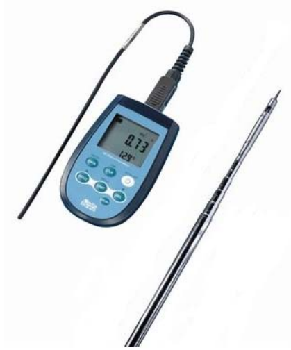
Figure 3.7. The HD 2303.0 anemometer used in the experiments to measure fluid velocity.
