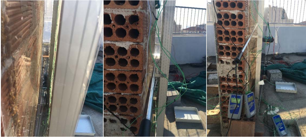
Figure 3.8. Hot wire anemometer probe inserted to a drilled hole on the plexiglass side of the experimental apparatus to measure the air velocity in the duct.
