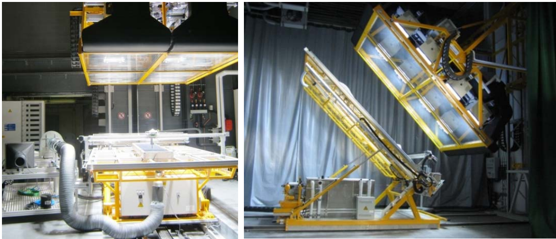
Figure 2.12. BIPV/T air collector tested horizontally and in 45° slope, in the solar simulator and air collector testing platform (Yang and Athienitis, 2014).
