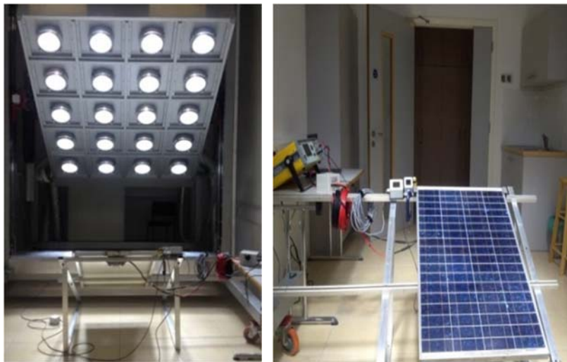
Figure 3.15. Experiment to obtain the characteristic curve of a PV indoors.
