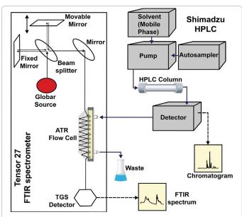
**Figure 1:** Schematic of the experimental layout of the coupled HPLC-FTIR technique. Chromatographic separations were performed by HPLC system using the Zorbax SB-Aq column. The mobile phase is then directed through a dedicated flow cell comprising a germanium ATR cell which was used for on-line FTIR detection.
