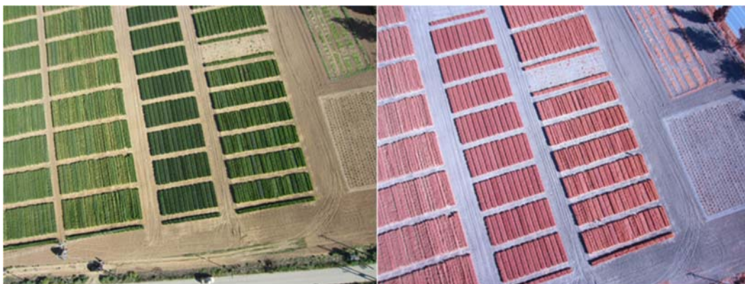
Figure 27: Sample photos from Canon IXUS 220 HS (left) and a modified near infrared Canon Powershot ELPH 300 HS (right).
