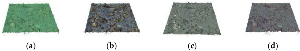
Figure 8. Medium quality point cloud for shallow waters dataset from the original imagery (a), the imagery corrected by the CLAHE based algorithm (b), the imagery corrected by the algorithm of Bianco et al., (2015) (c) and the imagery corrected with Adobe Photoshop (d).
