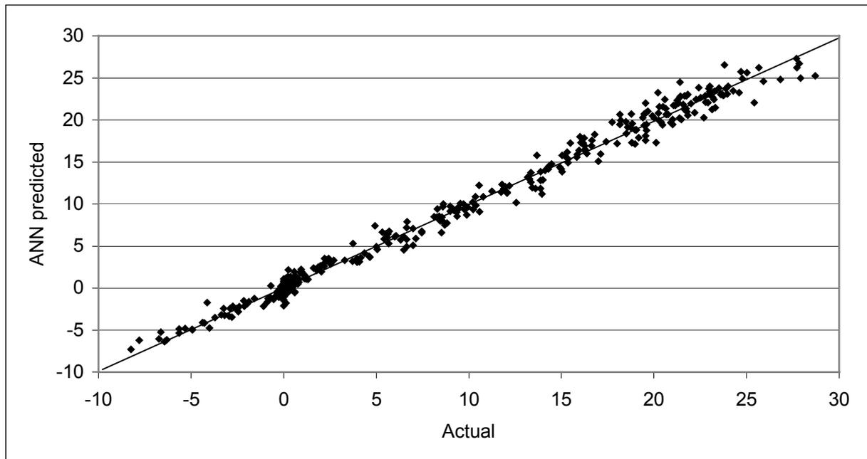
Figure 5. Comparison between the actual (modelled) and ANN predicted maximum loads for the validation data set.
