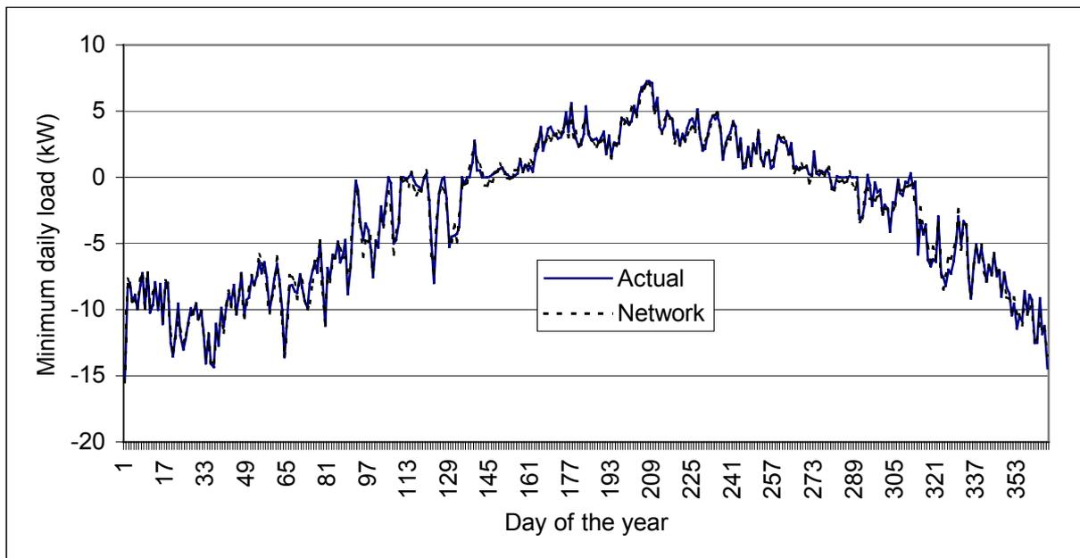
Figure 4. Comparison between the actual (modelled) and ANN predicted minimum load for the validation data set.
