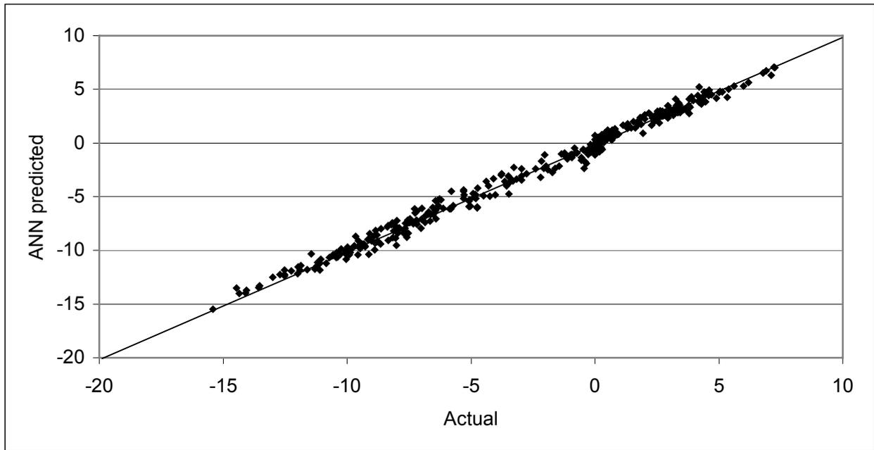
Figure 6. Comparison between the actual (modelled) and ANN predicted minimum loads for the validation data set.
