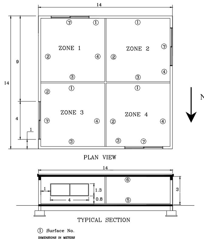
Figure 1. Drawing of the house modelled.
