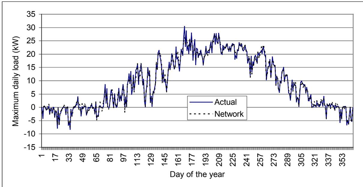
Figure 3. Comparison between the actual (modelled) and ANN predicted maximum load for the validation data set.
