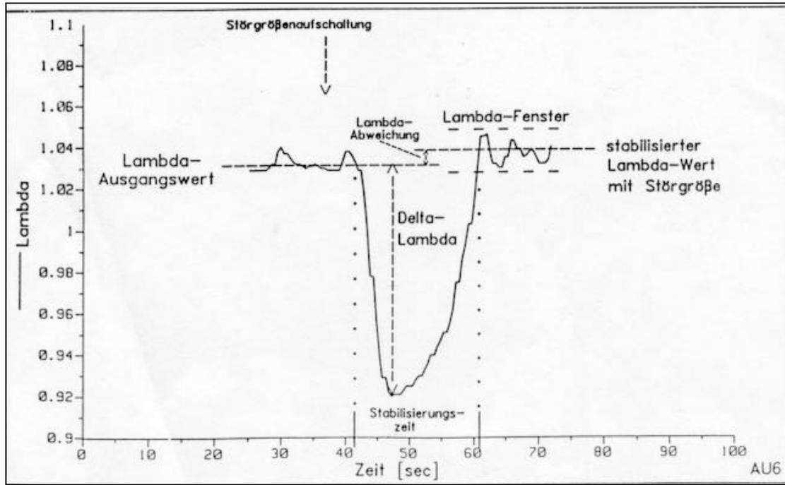
**Figure 1:** Example of artificial air/fuel ratio modification (Richter et al. 1993). When propane gas is added to the engine at  $t = 36$  s (“Störgrößenaufschaltung”), the engine switches to rich operation until the lambda control system restores a stabilised  $\lambda$  value (“stabilisierter Lambda-Wert mit Störgröße”) that slightly deviates from the initial one (“Lambda-Ausgangswert”); stabilisation time in this case is about 20 s.
