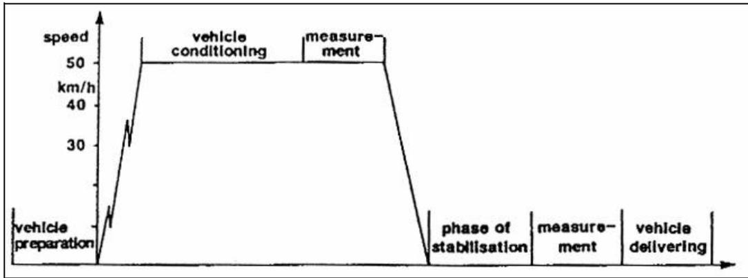
Figure 4: VdTÜV's short test for gasoline cars
