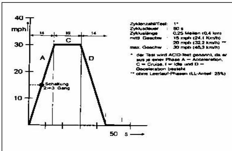
Figure 8: The New Jersey ACID Test
