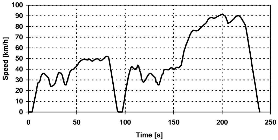
Figure 12: The IM 240 Test
