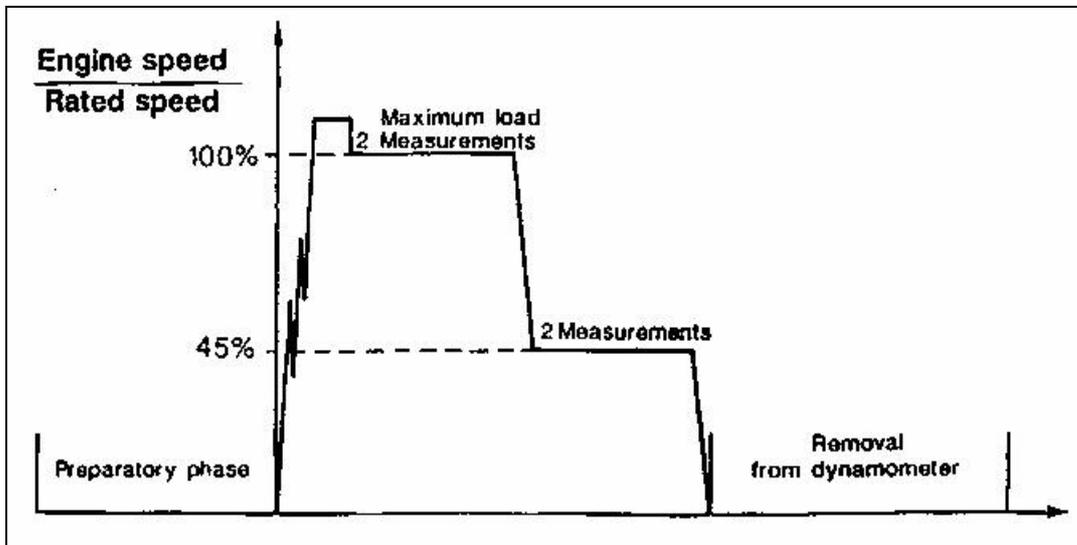
Figure 5: VdTÜV's short test for diesel cars
