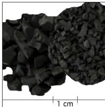
Figure 1-1: Recycled Tyre Rubber Particles
