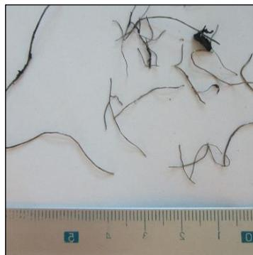
Figure 1-2 : Recycled Tyre Steel Fibres
