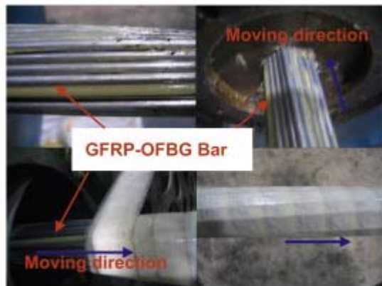
FRP-OFBG bars and steel wires twisted and passed through frames
