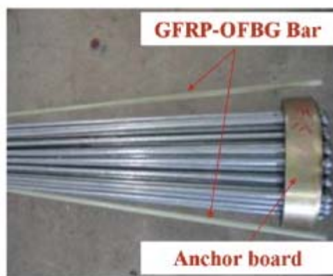
The exposed FRP-OFBG bars after PE sheaths decorticated
