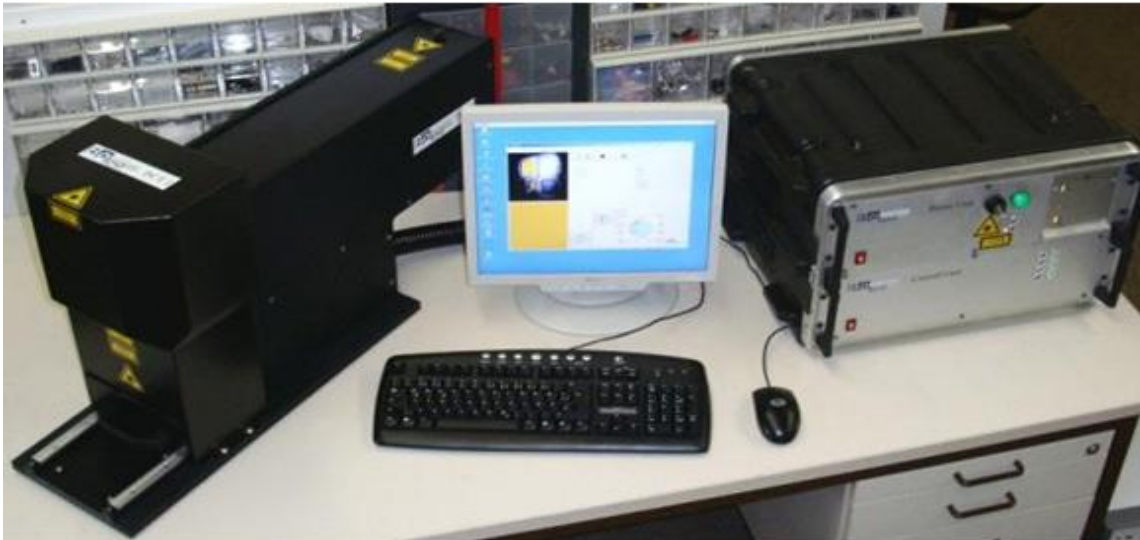
Image 8 : Photoelectrical System for examination of defects and aging effects of organic light emitting diodes (OLEDs) and organic and anorganic solar cells.(PCT1)
