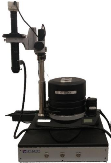
Figure 4-17: NT-MDT NTEGRA AFM, (RUNMS Characterization Lab, 2015)
