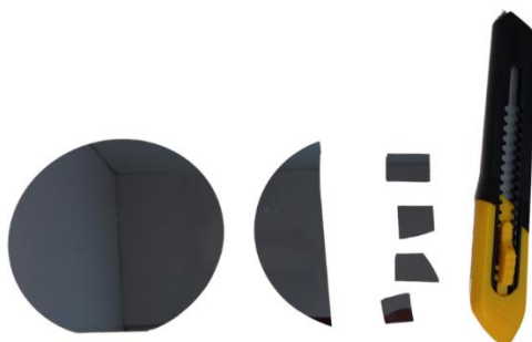
Figure 4-3: Si wafer and its pieces after been sliced using a cutter
