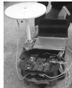
Fig. 11. Actual depiction of the system during an experiment. The FPGA, laptop and GPS antenna are clearly visible while the GPS receiver is under the laptop.
