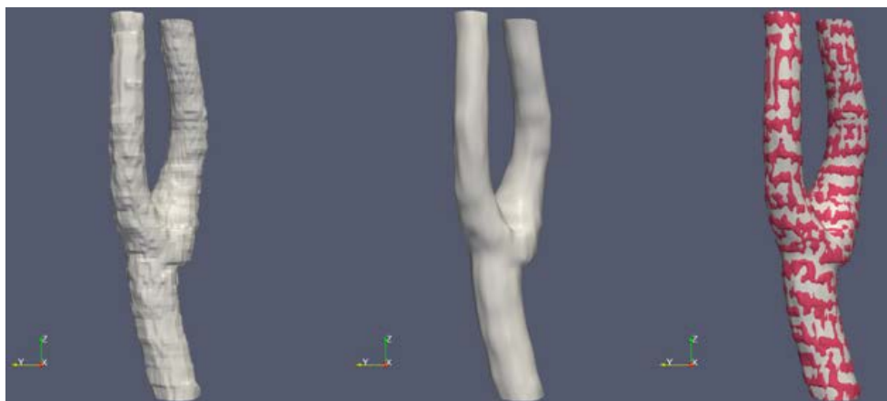
Figure 22: The initial constructed model (Left), the final smoothed model (middle), and the overlapping between initial and smooth model (right).
