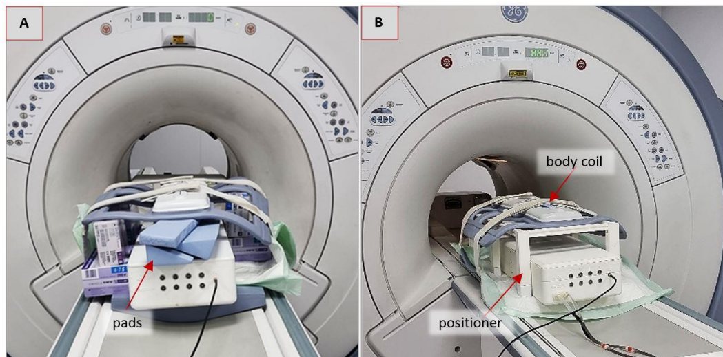
Figure 55: The robotic device positioned on the table of the 1.5 T MRI scanner, with the multi-channel body coil (A) placed directly above the phantom using pads and supporting objects and (B) securely mounted using a dedicated 3D printed plastic structure.
