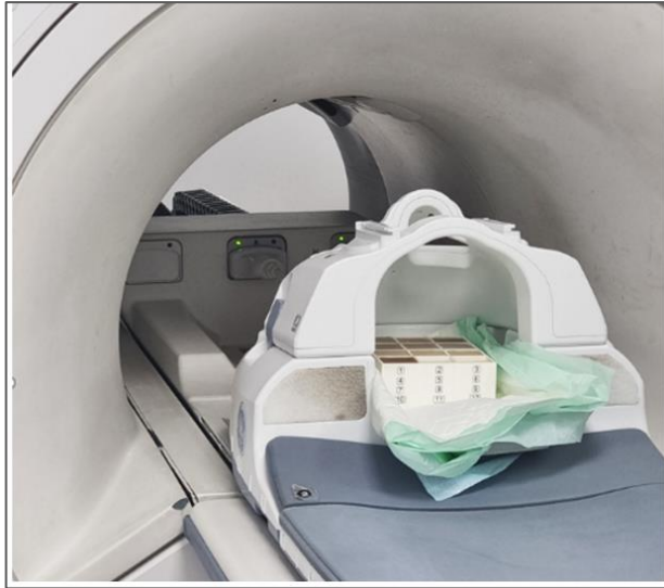
Figure 19: The phantom container positioned on the MRI table within the posterior head and face part of the head/neck/spine coil.
