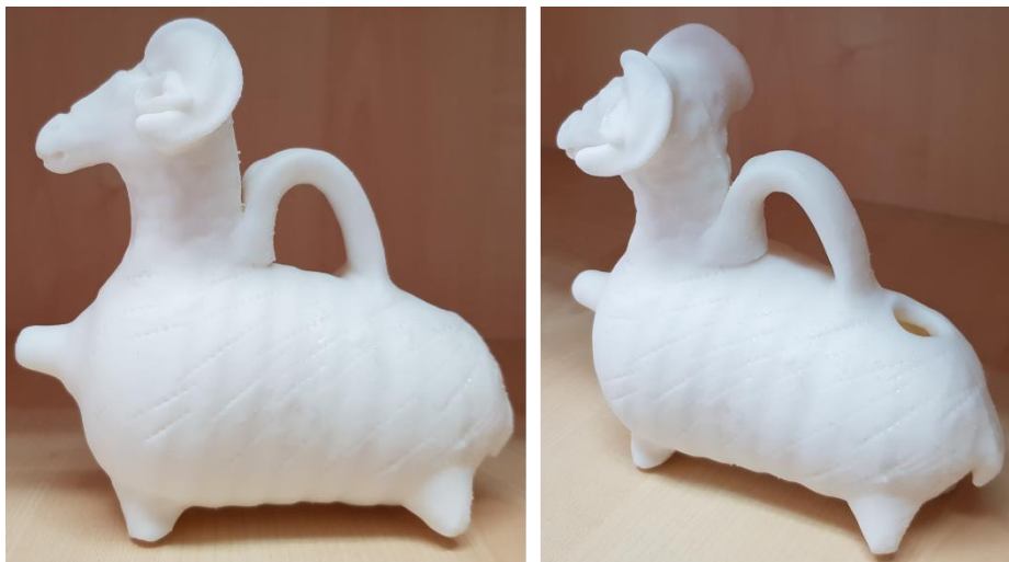
Figure 24: 3D printed replica of zoomorphic rhyton from CT scans.
