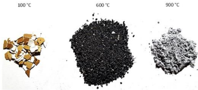
Figure 1-13. Eggshells rinsed with deionized water and dried at 100 °C, (b) calcinated at 600 °C for 3 h and (c) calcinated at 900 °C for 30 min (adapted from Panagiotou et al., 2018).
