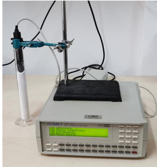
Figure 5.11.4: Experimental set-up in order to measure the thermal properties of the silicon dioxide and agar.
