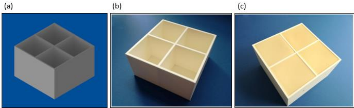
Figure 5.5.1: a) CAD drawing of the phantom mold (final version) which was used to produce 4 phantoms with different recipe for estimating the ultrasonic absorption coefficient, b) photo of the mold before filling the mixture, and c) after filling the mixture.
