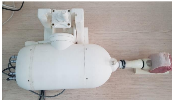
Figure 8.8.3.1: Experimental set-up with the excised tissue pierced and the probe inserted in the center of the tissue.
