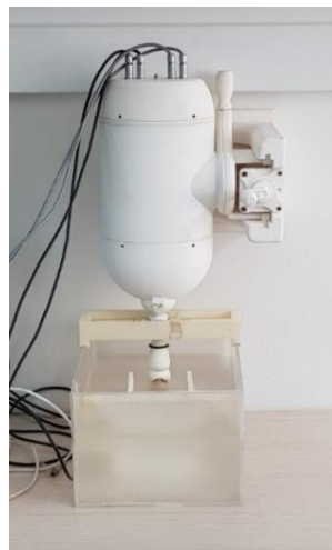
Figure 8.8.2.1: Experimental set-up when both the excised tissue and probe were immersed in degassed water.
